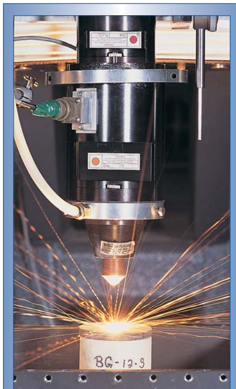
GTI is installing a 5-kW ytterbium fiber laser for use in its continuing research on the application of laser energy in well construction and completion.
