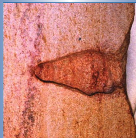
Figure 1. The Berea sandstone block is shown after perforation using the MIRACL laser. After perforation, measurements of permeability and acoustic properties were taken.
